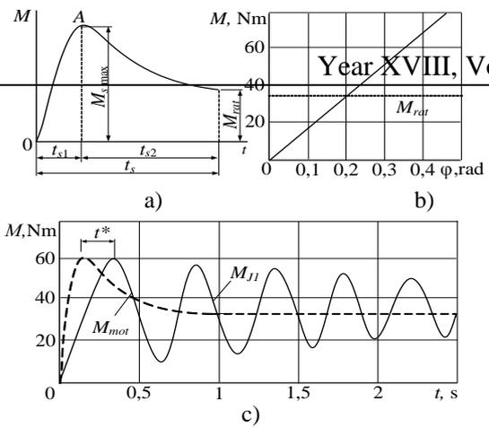
Figure 1. Modelling of oscillatory processes of transmission starting of a machine assembly: starting torque (a); linear elastic characteristic (b); oscillatory process of transmission starting of a machine assembly with a coupling that possesses linear elastic characteristic (c)
