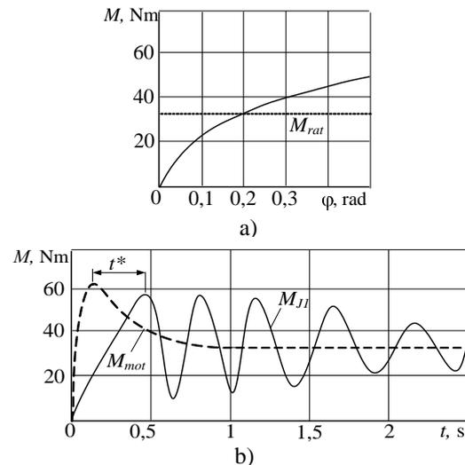
Figure 2. Oscillatory process of asynchronous motor starting: elastic characteristic of a "soft" Duffing type coupling (a); oscillatory process (b).
