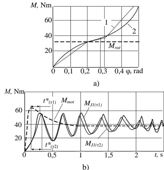
Figure. 4. Oscillatory process of asynchronous motor starting: combined elastic characteristics (a); oscillatory process (b).
