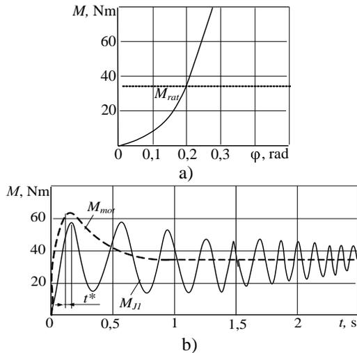
Figure. 3. Oscillatory process of asynchronous motor starting: elastic characteristic of a "hard" Duffing type coupling (a); oscillatory process (b).
