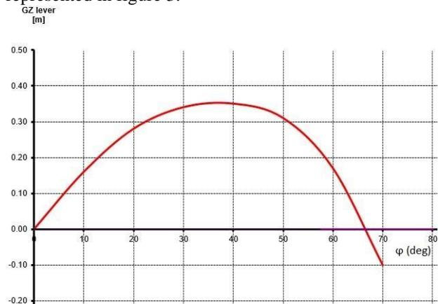
Figure 3 Illustration of righting arm curve for departure condition
