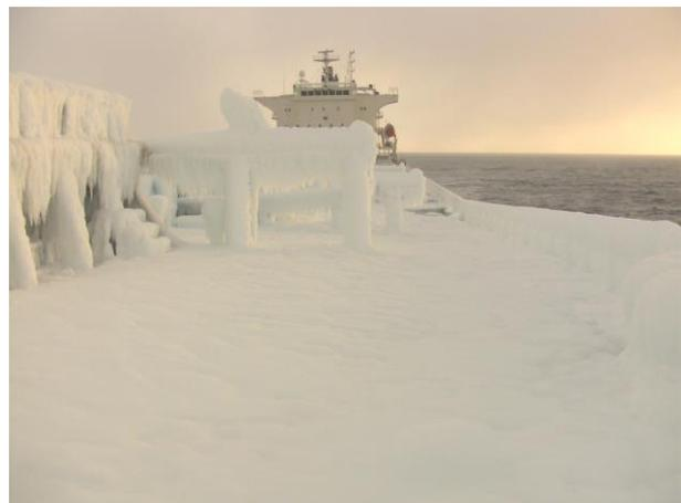
Figure 2 Large ice accumulations on board ship [source: author]
