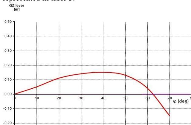
Figure 4 Illustration of righting arm curve for departure condition
