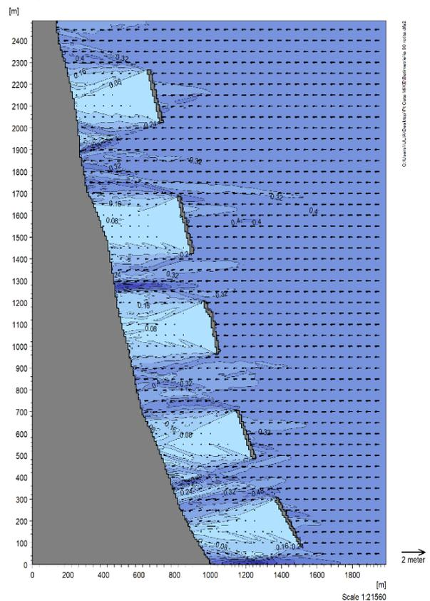
Figure 8 Wave height - Mamaia Bay with perpendicular incoming waves
