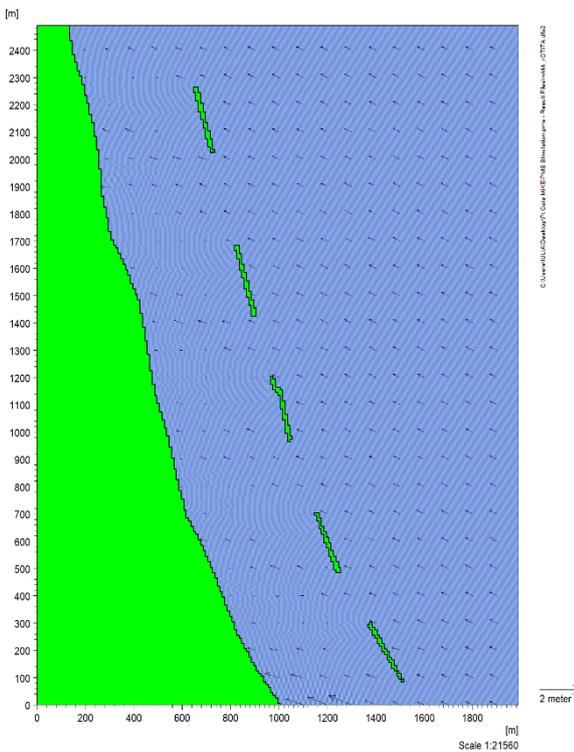
Figure 10 Refraction and diffraction of the Mamaia Bay with 129° incoming waves
