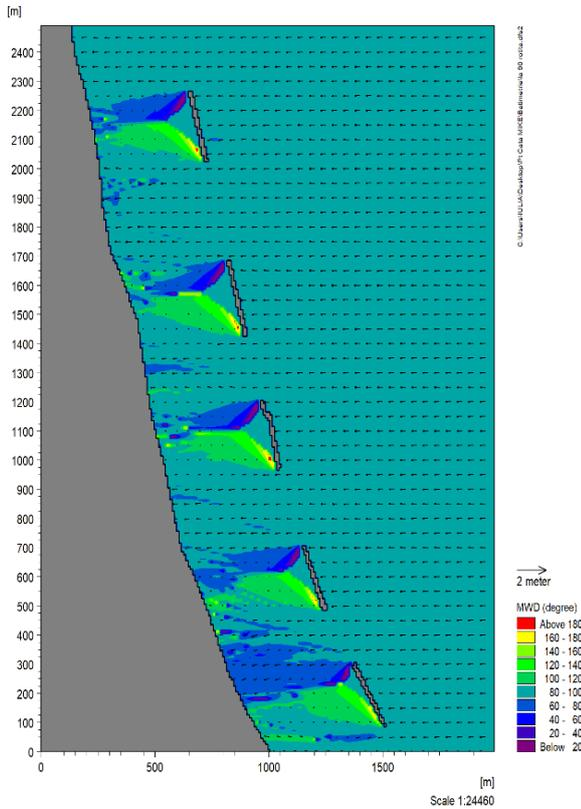
Figure 9 Direction of waves - Mamaia Bay with perpendicular incoming waves
