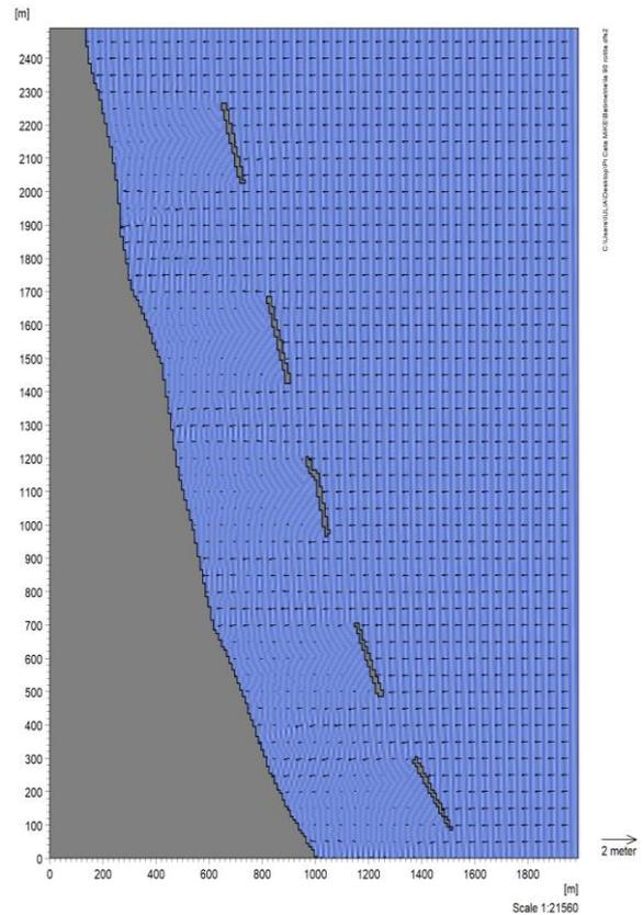
Figure 11 Refraction and diffraction of the Mamaia Bay with 129° incoming waves
