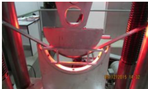
Figure 11 „U”shape forming process beginning
