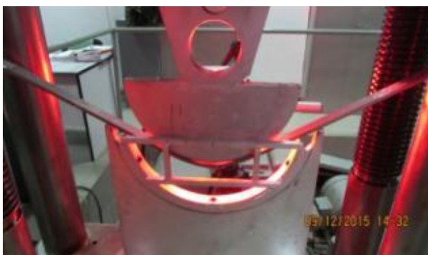
Figure 12 „U”shape forming process beginning
